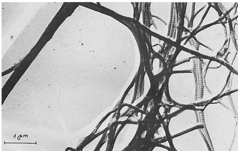
Fig. 7. Transmission electron microscopy (TEM) micrograph of unmodified chrome-tanned collagen fibers.
